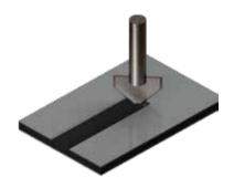
ALUPANEL can easily be folded by hand if a "V" shaped groove is milled on the rear of the panel. This can be done using a conventional router (available from your local DIY store) or CNC milling machine. A minimum of 0.30mm Polyethylene should be left on the back layer when routing to avoid sharp corners or paint chipping.
