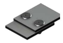
ALUPANEL can be riveted with standard equipment using rivets or blind rivets. For external use please refer to our Thermal Expansion document (available from your local Sales Manager/Distributor). Hole Size = Rivet Width +2mm
